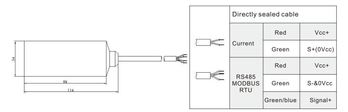
S=Signal, Vcc=Power Supply, GND=Vcc-&S-
