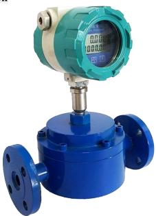
HEG oval wheel gear rotor flow meters are mainly used to measure high-viscosity media. The products are widely used in petroleum, petrochemical, natural gas, chemical, paper making and other industries to measure small flow meters with small diameters.
