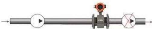
The sensor cannot be installed at the inlet of the pump. It can be installed at the outlet
