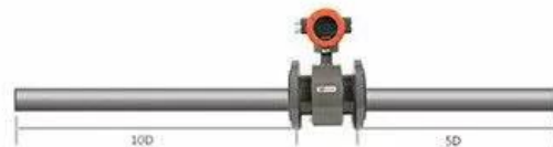
Need 10D of upstream and 5D of downstream
