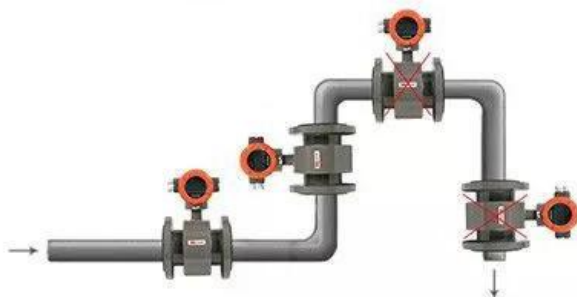
Install at the lowest point and vertical upward direction Don't install at the highest point and vertical downward direction
