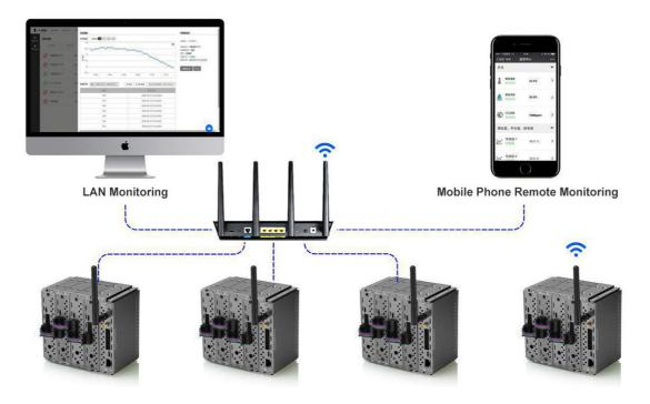
2. The combination of HW300 host and module connects to the system via Ethernet (wifi)
